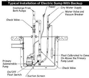
One type of a backup pump is powered by the water supply to the home. These have the advantage of being mechanically simple, relatively inexpensive and can do the job until you repair the primary pump or the power is restored. This pump does waste water, so they are not to be used as a primary pump, only a backup.
